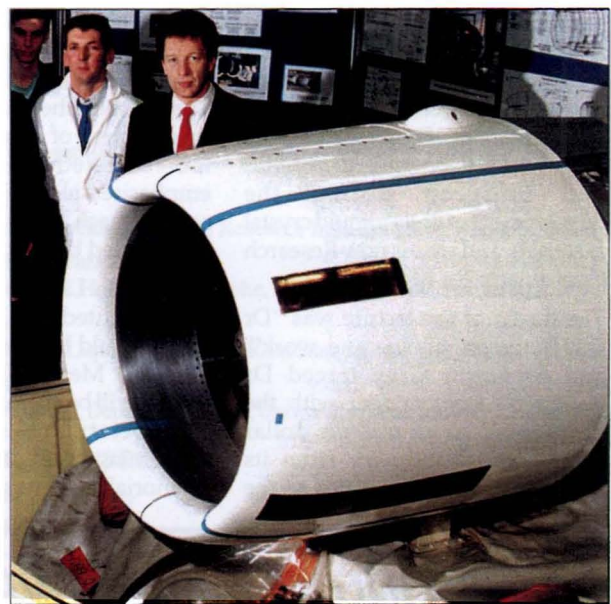
Fig 1: The jet engine nacelle to be tested in the European Laminar Flow Flight Demonstrator Programme. The liquid crystal heater section can be seen as the lower and larger of the two dark strips on the nacelle.
